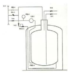
is (V-3) adequate for the intended application. If additional pressurization is required, open the pressure-building valve to operate the integral pressure-building coil (PBC-1). With the pressure-building system functioning, the preset pressure will be maintained throughout the withdrawal as long as a sufficient liquid supply is present.
